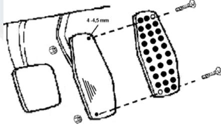
The clutch and brake pedal cover are installed as follows.
