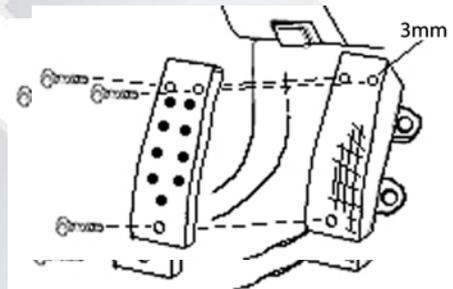
Hold the pedal plate to the accelerator pedal and mark the mounting holes. With a 4 - 4,5 mm drill bit, drill holes on the marked positions. Install the plate with the supplied fittings.
